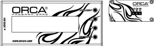
Connect the battery wires to a charged pack of battery. Turn on the ESC and the setting card will activate automatically. Note that the screen will show "Loading..." during initialization – indicating that the ESC is copying the current setup in the ESC to the setting card. Once loading is completed, the screen will show "ORCA VRITRA-VTC - Program". You can now start to program your ESC.
