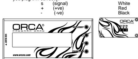
Connect the battery wires to a charged pack of battery. Turn on the ESC and the setting card will activate automatically. Note that the screen will show "Loading..." during initialization - indicating that the ESC is copying the current setup in the ESC to the setting card. Once loading is completed, the screen will show "TEAM ORCA Program" and Current Firmware Version and Data code e.g. Ver3.0 1XXXXXA. You can now start to program your ESC.
