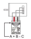
A+B-C must match the initial setup or match your programming setup. (WARNING! Improper configuration may damage the ESC.)
