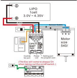
\*Install/Solder the relevant battery connector (Battery Specific) to the battery wires. Red to +ve and Black to -ve. (The ESC has no response when reverse the +ve and -ve) \* Connect supplied BEC wire(200mm) to 3pin port match the (+ s) between the
