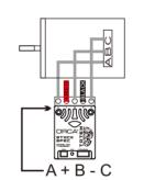
A+B-C must match the initial setup or match your programming setup.(WARNING! Improper configuration may damage the ESC.)
