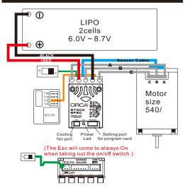
Red to +ve and Black to -ve. (The ESC has no response when reverse the +ve and -ve) \* Connect supplied BEC wire(200mm) to 3pin port match the (- + s) between the receiver connector and ESC
